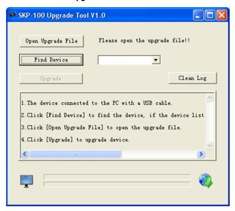
Click "Find Device", If the device list is empty, reconnect SKP-100 or to install the driver.
