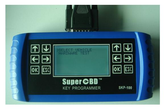
Press [OK] to enter the vehicle selection. Press the arrow keys to select vehicles.
